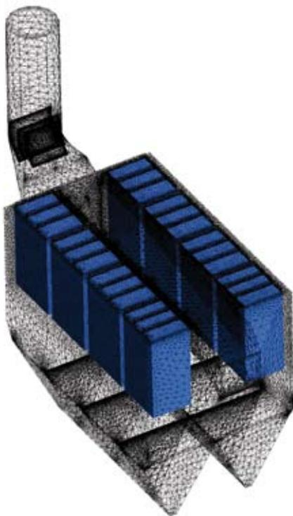
3D model of an electrostatic filter following conversion to ProJet mega® bag filter
